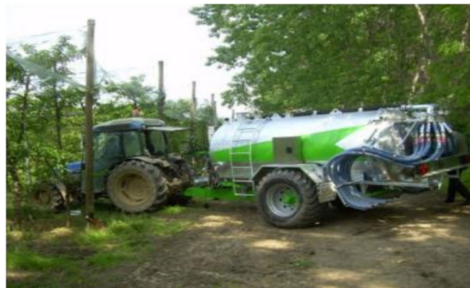
Fig. 2 Prototype slurry spreader with band application distribution system [45]
