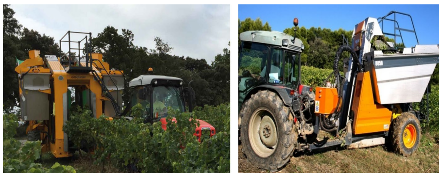
Fig. 8 Towed-type grape harvesters; a ) G3.220 ( https://www.gregoire.fr/en-oc/ ); b ) Grapes'Line ( https://pellenc.com/au/ )
