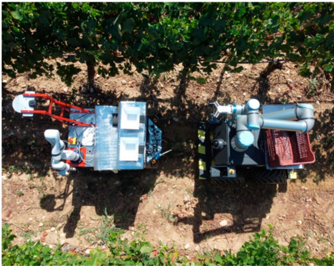
Fig. 12 Helper robot followed by expert robot, ready to support harvesting [84]
