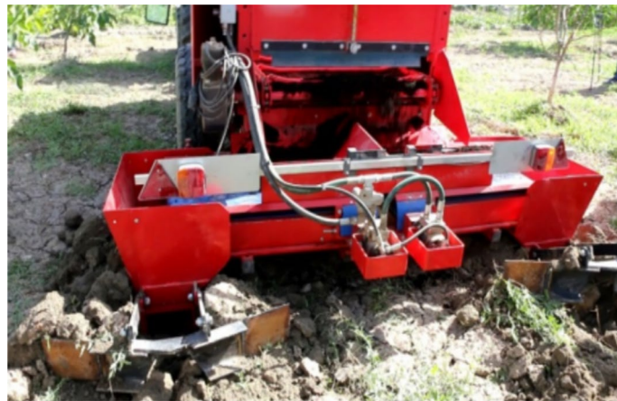
Fig. 1 Double ditches fertilizing device operating into the soil [44]
