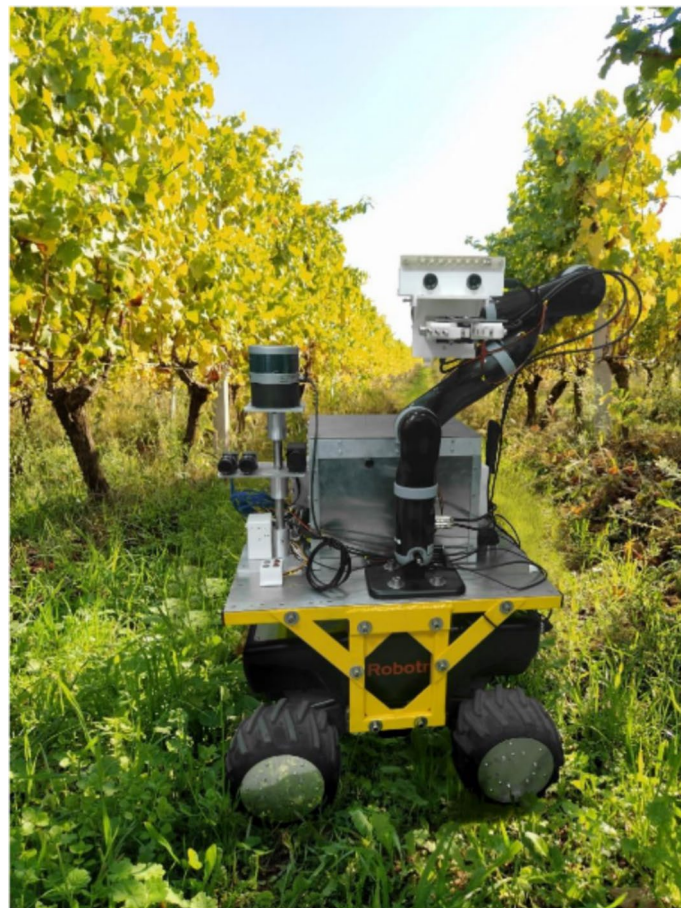
Fig. 11 Autonomous grape-harvester robot [82]
