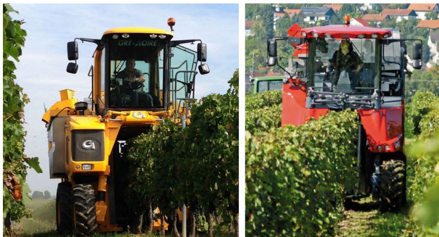
Fig. 7 Self-propelled grape harvesters; a ) Gregoire G7.200 ( https://www.gregoire.fr/en-oc/ ); b ) ERO-Grapeliner 6000 ( http://www.ero-viti.com/ )
