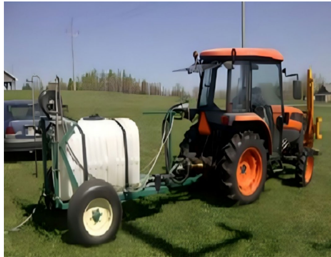
Fig. 3 Biochar slurry applicator for grape vines [47]
