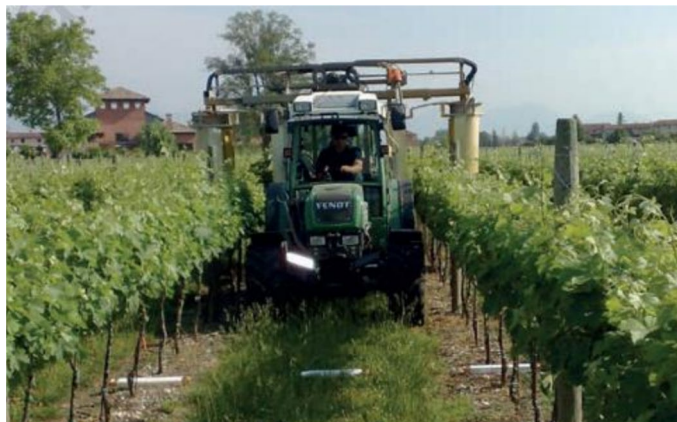
Fig. 5 Tunnel sprayer during operation in vineyards [52]
